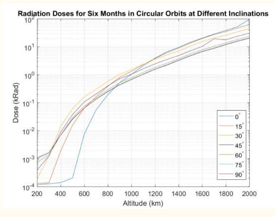
Dose values are for a spacecraft modeled with 0.7mm of Aluminum shielding.
