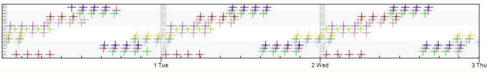
Coverage of satellites after they've been propagated for 6 months with all the perturbations. Resulted in continuous coverage from BOL to EOL.
